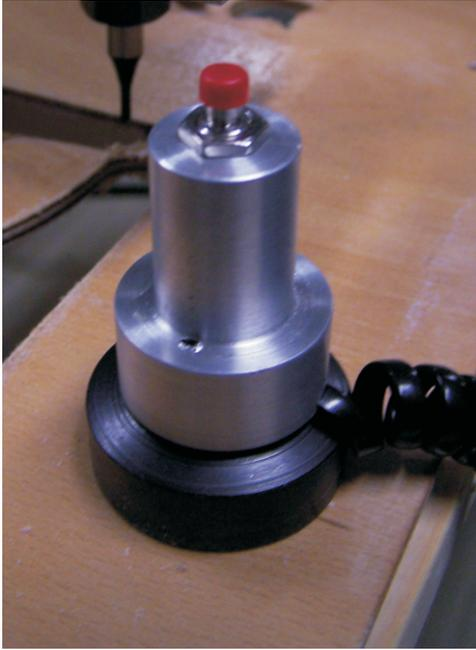
The sensor is a mechanical or electronic or optical sensor, which has set the exact length of the switch. This is then used during the start-up material (workpiece), the second way, running into the material by hand according to the eye.
